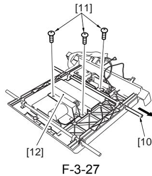
6) Disconnect all connector from the shift tray driver PCB.
